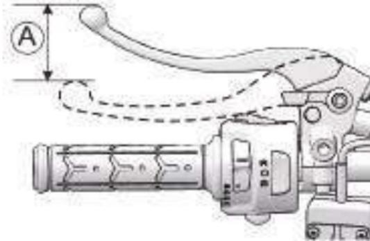
1. Squeeze the parking brake lever with force, squeeze and release the action, repeat a few times, the parking brake lever shall not be stuck.
