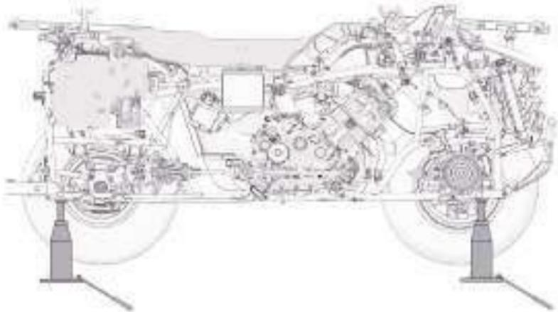
**Schematic diagram of jack support position**
