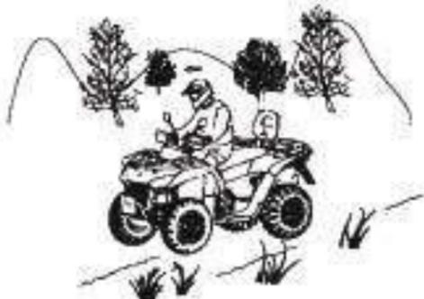
4. If the vehicle begins to tip, quickly turn the front wheel downhill, if possible, or dismount on the uphill side immediately!
