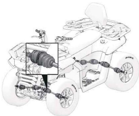
Check the front and rear drive shaft boots for cuts, cracks, damage or grease leaks. If so, contact your Segway dealer for a replacement.
