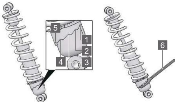
1. There are 5 shock absorption positions, which are used for different loads or driving conditions.
