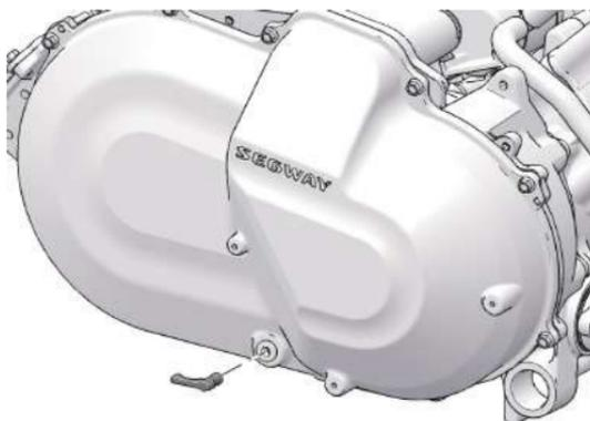
1. Remove the clutch drain plug.
