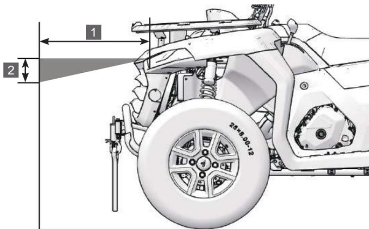
2. Measure the distance from the floor to the center of the headlights and mark the walls at the same height.
