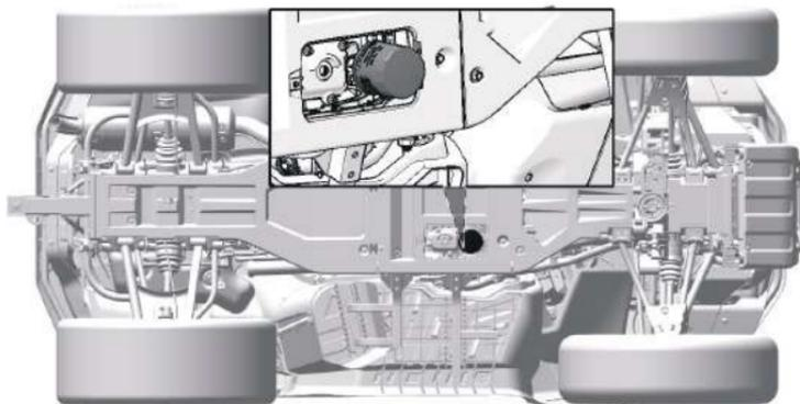
1. Remove the screw of the frame bottom maintenance cover plate, remove the frame bottom maintenance cover plate, the oil filter is located here, put the towel under the oil filter.
