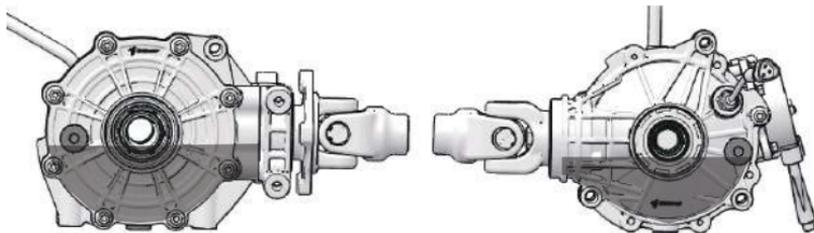
1. Position the vehicle on a horizontal surface and remove the filling plug.
