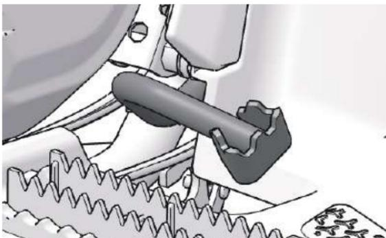
The foot brake is the main brake system of the vehicle. The main brake is located on the right foot plate of the vehicle. When the vehicle needs to slow down or stop, step on the foot brake slowly. Emergency braking can cause the vehicle to skid or roll over, so do not use emergency braking when it is not necessary.
