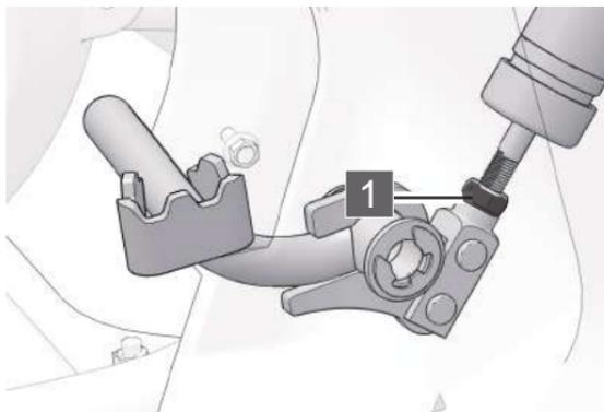
The foot brake lever adjusting nut is located at the bottom of the vehicle near the foot brake lever. The stroke height of the foot brake lever can be adjusted by twisting the foot brake lever nut.
